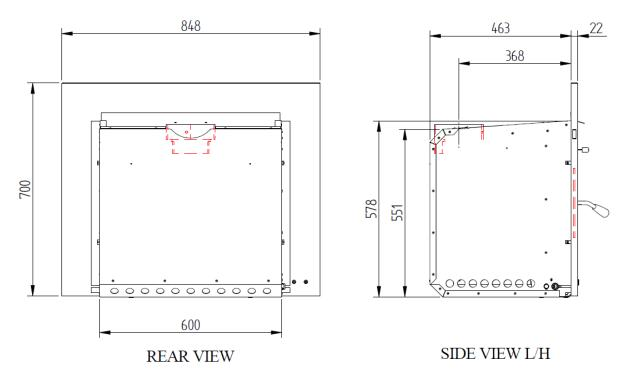
NOTE: Dimensions do not include the insulating blanket. Add 15mm to rear and top to allow for insulating blanket.
