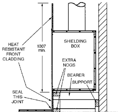
**Fig. 4 ELEVATED INSTALLATION**
